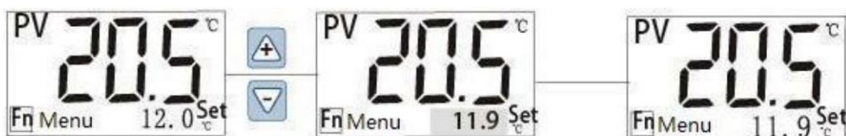
To change the set temperature of the chiller, while on the main interface press the "Up" or "Down" arrow to change the displayed set temperature.
